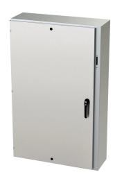
Saginaw Enviroline series disconnect enclosure, NEMA 3R/4/4X/12/13, right flange, 60 x 37 x 12in (HxWxD), wall mount, 304 stainless steel, #4 brush finish, single-door, 3-point padlocking handle, purchase subpanel separately.
