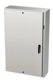
Saginaw Enviroline series disconnect enclosure, NEMA 3R/4/4X/12/13, right flange, 60 x 37 x 12in (HxWxD), wall mount, 316L stainless steel, #4 brush finish, single-door, 3-point padlocking handle, purchase subpanel separately.
