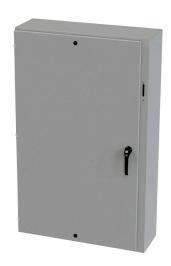
Saginaw Enviroline series disconnect enclosure, NEMA 3R/4/12/13, right flange, 60 x 37 x 12in (HxWxD), wall mount, carbon steel, ANSI 61 gray, powder coat finish, single-door, 3-point padlocking handle, purchase subpanel separately.
