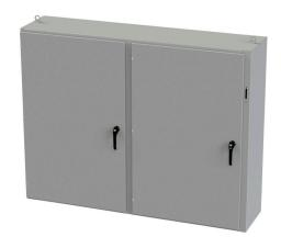
Saginaw disconnect enclosure, NEMA 3R/12/13, right flange, 60 x 78 x 18in (HxWxD), freestanding/wall-mount, carbon steel, ANSI 61 gray, powder coat finish, 2-door, 3-point padlocking handle, purchase subpanel separately.
