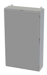
Saginaw enclosure, NEMA 3R/4/12/13, 60 x 36 x 12in (HxWxD), wall mount, carbon steel, ANSI 61 gray, powder coat finish, single-door, plated steel clamps, padlock hasp and staple.
