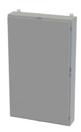
Saginaw enclosure, NEMA 3R/4/12/13, 60 x 36 x 8in (HxWxD), wall mount, carbon steel, ANSI 61 gray, powder coat finish, single-door, plated steel clamps, padlock hasp and staple.
