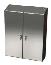
Saginaw Enviroline series enclosure, slope top, NEMA 3R/4/4X/12/13, 60 x 60 x 18in (HxWxD), freestanding, 304 stainless steel, #4 brush finish, 2-door, 3-point 304 stainless steel padlocking handle.
