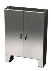
Saginaw Enviroline series enclosure, NEMA 3R/4/4X/12/13,  $60 \times 60 \times 18$ in (HxWxD), floor mount, 304 stainless steel, #4 brush finish, 2-door, 3-point keylocking/padlocking combo handle.
