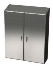
Saginaw Enviroline series enclosure, slope top, NEMA 3R/4/4X/12/13,  $60 \times 60 \times 18$  in (HxWxD), freestanding, 316L stainless steel, #4 brush finish, 2-door, 3-point 304 stainless steel padlocking handle.
