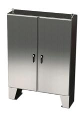
Saginaw Enviroline series enclosure, NEMA 3R/4/4X/12/13, 60 x 60 x 18in (HxWxD), floor mount, 316L stainless steel, #4 brush finish, 2-door, 3-point keylocking/padlocking combo handle.
