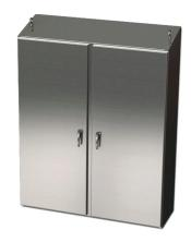
Saginaw Enviroline series enclosure, slope top, NEMA 3R/4/4X/12/13, 60 x 60 x 12in (HxWxD), freestanding, 304 stainless steel, #4 brush finish, 2-door, 3-point 304 stainless steel padlocking handle.
