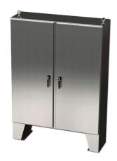
Saginaw Enviroline series enclosure, NEMA 3R/4/4X/12/13, 60 x 60 x 12in (HxWxD), floor mount, 304 stainless steel, #4 brush finish, 2-door, 3-point keylocking/padlocking combo handle.
