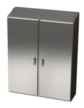
Saginaw Enviroline series enclosure, slope top, NEMA 3R/4/4X/12/13,  $60 \times 60 \times 12$  in (HxWxD), freestanding, 316L stainless steel, #4 brush finish, 2-door, 3-point 304 stainless steel padlocking handle.
