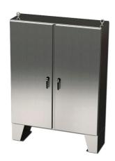
Saginaw Enviroline series enclosure, NEMA 3R/4/4X/12/13, 60 x 60 x 12in (HxWxD), floor mount, 316L stainless steel, #4 brush finish, 2-door, 3-point keylocking/padlocking combo handle.
