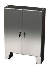
Saginaw Enviroline series enclosure, NEMA 3R/4/4X/12/13, 60 x 48 x 18in (HxWxD), floor mount, 304 stainless steel, #4 brush finish, 2-door, 3-point keylocking/padlocking combo handle.
