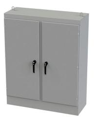
Saginaw Enviroline series enclosure, NEMA 3R/4/12/13, 60 x 48 x 18in (HxWxD), freestanding, carbon steel, ANSI 61 gray, powder coat finish, 2-door, 3-point keylocking/padlocking combo handle.
