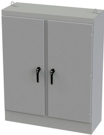
Saginaw Enviroline series enclosure, NEMA 3R/4/12/13, 60 x 48 x 18in (HxWxD), freestanding, carbon steel, ANSI 61 gray, powder coat finish, 2-door, 3-point keylocking/padlocking combo handle.
