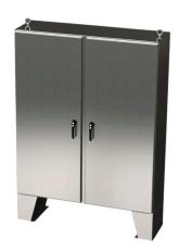
Saginaw Enviroline series enclosure, NEMA 3R/4/4X/12/13, 60 x 48 x 12in (HxWxD), floor mount, 304 stainless steel, #4 brush finish, 2-door, 3-point keylocking/padlocking combo handle.
