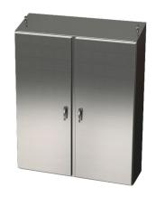
Saginaw Enviroline series enclosure, slope top, NEMA 3R/4/4X/12/13, 60 x 48 x 12in (HxWxD), freestanding, 316L stainless steel, #4 brush finish, 2-door, 3-point 304 stainless steel padlocking handle.
