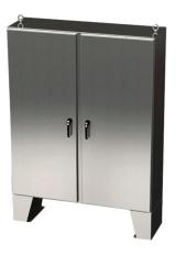
Saginaw Enviroline series enclosure, NEMA 3R/4/4X/12/13, 60 x 48 x 12in (HxWxD), floor mount, 316L stainless steel, #4 brush finish, 2-door, 3-point keylocking/padlocking combo handle.
