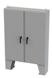
Saginaw Enviroline series enclosure, NEMA 3R/4/12/13, 60 x 48 x 12in (HxWxD), floor mount, carbon steel, ANSI 61 gray, powder coat finish, 2-door, 3-point keylocking/padlocking combo handle.
