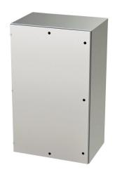
Saginaw Enviroline series enclosure, NEMA 3R/4/4X/12/13, 60 x  $36 \times 24$ in (HxWxD), wall mount, 304 stainless steel, #4 brush finish, single-door, 1/4-turn semi-flush latch.
