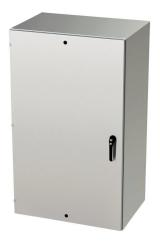
Saginaw Enviroline series enclosure, NEMA 3R/4/4X/12/13, 60 x 36 x 24in (HxWxD), wall mount, 304 stainless steel, #4 brush finish, single-door, 3-point keylocking/padlocking combo handle.
