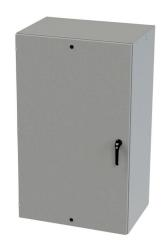
Saginaw Enviroline series enclosure, NEMA 3R/4/12/13, 60 x 36 x 24in (HxWxD), wall mount, carbon steel, ANSI 61 gray, powder coat finish, single-door, 3-point keylocking/padlocking combo handle.
