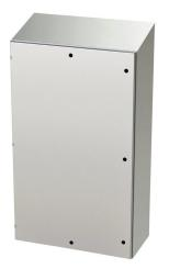
Saginaw Enviroline series enclosure, slope top, NEMA 3R/4/4X/12/13, 60 x 36 x 16in (HxWxD), wall mount, 304 stainless steel, #4 brush finish, single-door, 1/4-turn semi-flush latch.
