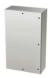
Saginaw Enviroline series enclosure, NEMA 3R/4/4X/12/13, 60 x 36 x 16in (HxWxD), wall mount, 304 stainless steel, #4 brush finish, single-door, 1/4-turn semi-flush latch.
