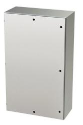
Saginaw Enviroline series enclosure, NEMA 3R/4/4X/12/13, 60 x 36 x 16in (HxWxD), wall mount, 316L stainless steel, #4 brush finish, single-door, 1/4-turn semi-flush latch.
