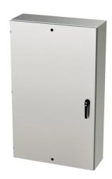
Saginaw Enviroline series enclosure, NEMA 3R/4/4X/12/13, 60 x  $36 \times 12$  in (HxWxD), wall mount, 316L stainless steel, #4 brush finish, single-door, 3-point keylocking/padlocking combo handle.
