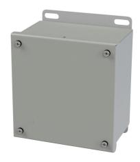
Saginaw enclosure, NEMA 3R/4/12/13, 6 x 6 x 4in (HxWxD), wall mount, carbon steel, ANSI 61 gray, powder coat finish, screw cover.
