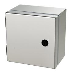
Saginaw Enviroline Junction series enclosure, NEMA 3R/4/4X/12/13, 6 x 6 x 4in (HxWxD), wall mount, 304 stainless steel, #4 brush finish, single-door, 1/4-turn semi-flush latch.
