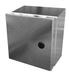
Saginaw Enviroline Junction series enclosure, slope top, NEMA 3R/4/4X/12/13, 6 x 6 x 4in (HxWxD), wall mount, 304 stainless steel, #4 brush finish, single-door, 1/4-turn semi-flush latch.
