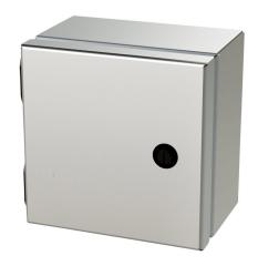
Saginaw Enviroline Junction series enclosure, NEMA 3R/4/4X/12/13, 6 x 6 x 4in (HxWxD), wall mount, 316L stainless steel, #4 brush finish, single-door, 1/4-turn semi-flush latch.
