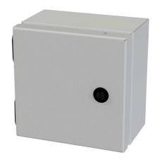
Saginaw Enviroline Junction series enclosure, NEMA 3R/4/12/13, 6 x 6 x 4in (HxWxD), wall mount, carbon steel, RAL 7035 light gray, powder coat finish, single-door, 1/4-turn semi-flush latch.
