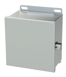
Saginaw enclosure, NEMA 3R/4/4X/12/13, 6 x 6 x 4in (HxWxD), wall mount, 304 stainless steel, #4 brush finish, single-door, stainless steel clamps.
