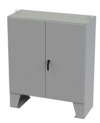
Saginaw enclosure, NEMA 3R/12/13, 60 x 60 x 24in (HxWxD), floor mount, carbon steel, ANSI 61 gray, powder coat finish, double-door, 3-point keylocking/padlocking combo handle.
