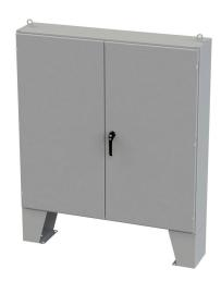
Saginaw enclosure, NEMA 3R/12/13, 60 x 60 x 12in (HxWxD), floor mount, carbon steel, ANSI 61 gray, powder coat finish, double-door, 3-point keylocking/padlocking combo handle.
