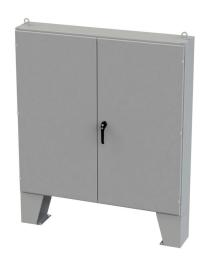
Saginaw enclosure, NEMA 3R/12/13, 60 x 60 x 10in (HxWxD), floor mount, carbon steel, ANSI 61 gray, powder coat finish, double-door, 3-point keylocking/padlocking combo handle.
