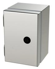
Saginaw Enviroline Junction series enclosure, NEMA 3R/4/4X/12/13, 6 x 4 x 4in (HxWxD), wall mount, 304 stainless steel, #4 brush finish, single-door, 1/4-turn semi-flush latch.
