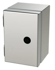
Saginaw Enviroline Junction series enclosure, NEMA 3R/4/4X/12/13, 6 x 4 x 4in (HxWxD), wall mount, 316L stainless steel, #4 brush finish, single-door, 1/4-turn semi-flush latch.
