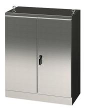
Saginaw enclosure, NEMA 3R/12/13, 60 x 48 x 18in (HxWxD), freestanding, 304 stainless steel, #4 brush finish, double-door, 3-point keylocking/padlocking combo handle.
