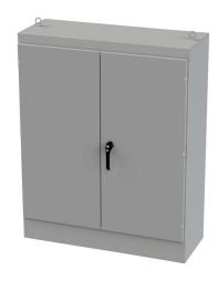
Saginaw enclosure, NEMA 3R/12/13, 60 x 48 x 18in (HxWxD), freestanding, carbon steel, ANSI 61 gray, powder coat finish, double-door, 3-point keylocking/padlocking combo handle.
