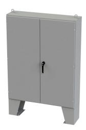
Saginaw enclosure, NEMA 3R/12/13, 60 x 48 x 12in (HxWxD), floor mount, carbon steel, ANSI 61 gray, powder coat finish, double-door, 3-point keylocking/padlocking combo handle.
