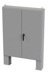
Saginaw enclosure, NEMA 3R/12/13, 60 x 48 x 8in (HxWxD), floor mount, carbon steel, ANSI 61 gray, powder coat finish, double-door, 3-point keylocking/padlocking combo handle.
