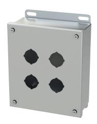
Saginaw pushbutton enclosure, 4 holes, 30mm, NEMA 4/4X/12/13, 8 x 7 x 3in (HxWxD), wall mount, 304 stainless steel, #4 brush finish, screw cover.
