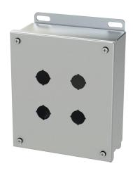
Saginaw pushbutton enclosure, 4 holes, 22mm, NEMA 4/4X/12/13, 8 x 7 x 3in (HxWxD), wall mount, 304 stainless steel, #4 brush finish, screw cover.
