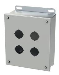
Saginaw pushbutton enclosure, 4 holes, 30mm, NEMA 4/4X/12/13, 8 x 7 x 3in (HxWxD), wall mount, 316L stainless steel, #4 brush finish, screw cover.
