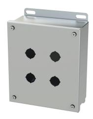
Saginaw pushbutton enclosure, 4 holes, 22mm, NEMA 4/4X/12/13, 8 x 7 x 3in (HxWxD), wall mount, 316L stainless steel, #4 brush finish, screw cover.
