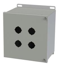
Saginaw pushbutton enclosure, 4 holes, 30mm, NEMA 4/12/13, 8 x 8 x 6in (HxWxD), wall mount, carbon steel, ANSI 61 gray, powder coat finish, hinged screw cover.
