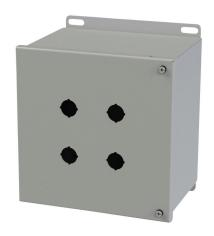
Saginaw pushbutton enclosure, 4 holes, 22mm, NEMA 4/12/13, 8 x 8 x 6in (HxWxD), wall mount, carbon steel, ANSI 61 gray, powder coat finish, hinged screw cover.
