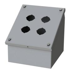
Saginaw pushbutton consolet, 4 holes, 30mm, NEMA 4/12/13, 7 x 7 x 7in (HxWxD), wall mount, carbon steel, ANSI 61 gray, powder coat finish, screw cover, purchase subpanel separately.
