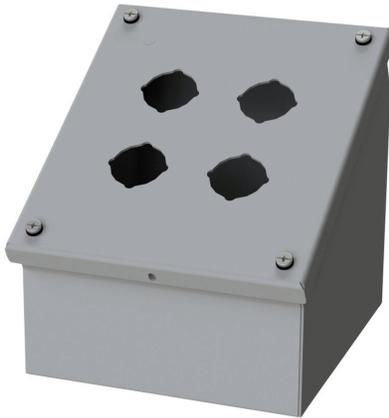
Saginaw pushbutton console, 4 holes, 30mm, NEMA 4/12/13, 7 x 7 x 7in (HxWxD), wall mount, carbon steel, ANSI 61 gray, powder coat finish, screw cover, purchase subpanel separately.
