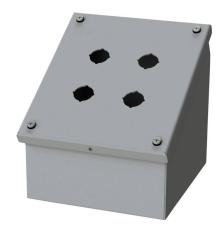
Saginaw pushbutton consolet, 4 holes, 22mm, NEMA 4/12/13, 7 x 7 x 7in (HxWxD), wall mount, carbon steel, ANSI 61 gray, powder coat finish, screw cover, purchase subpanel separately.
